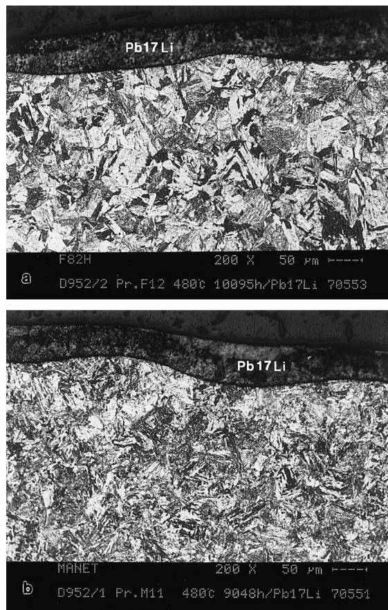
Fig. 2. Etched cross-sections of (a) F82H-mod. exposed for 10000 h and (b) MANET I exposed for 9000 h in Pb–17Li at 480°C.
